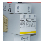
Surge protectors Class II overvoltage protectors – 1000V Class I+II – 1500V (EN 61643-31). Phase connection on top and earth connection on bottom. Module end of life visual indication
